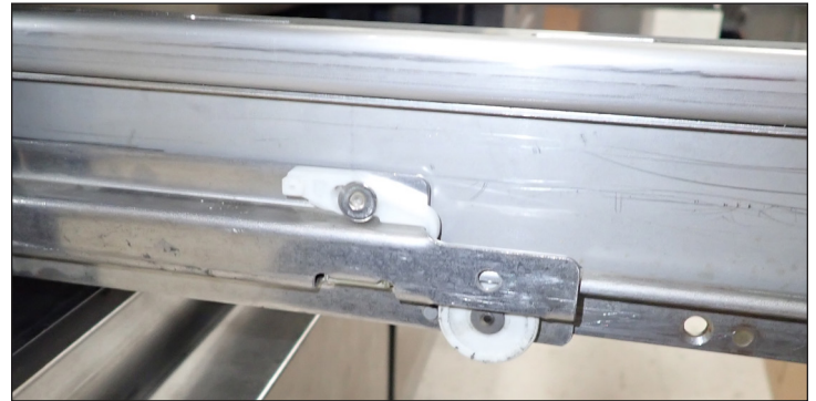
Fig. 1. Drawer retainer location. Retainer is engaged.
