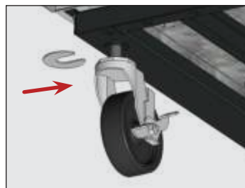
Fig. 9. Insert the castor shim(s). be sure to tighten the castor stem.
