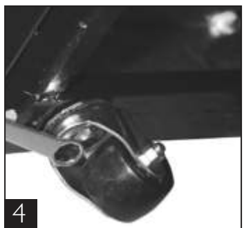
Tighten castor in position with castor wrench.
