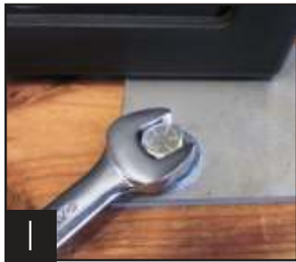
Removing bracket from skid.
