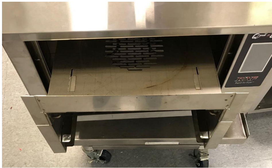
Air Plenum Pulled Out of the RAF
