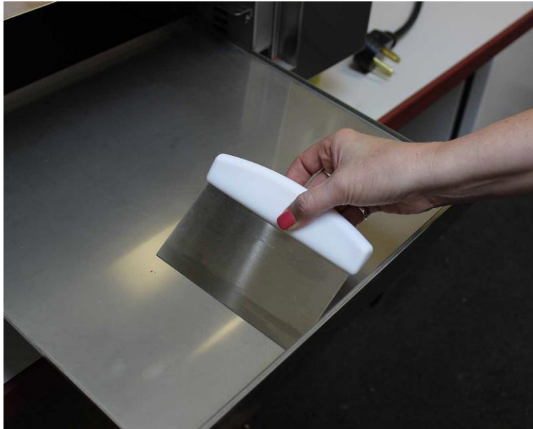
Scraping the Drip Tray to Clean
