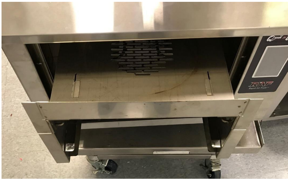
Air Plenum Pulled Out of the RAF
