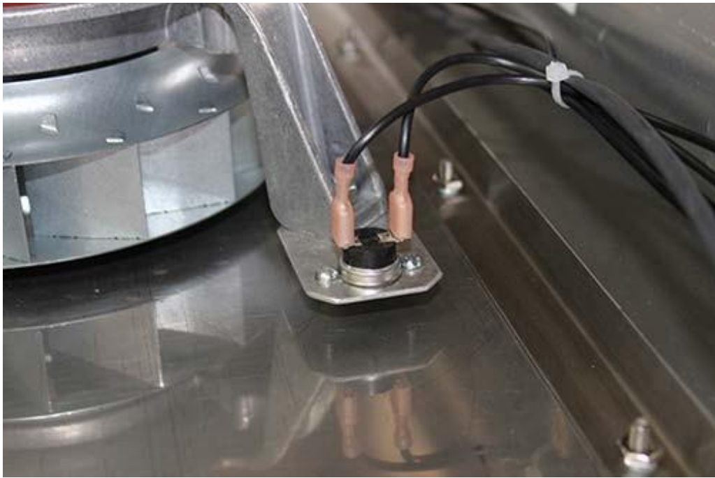
Top Oven Compartment Thermostat set to 145°F
