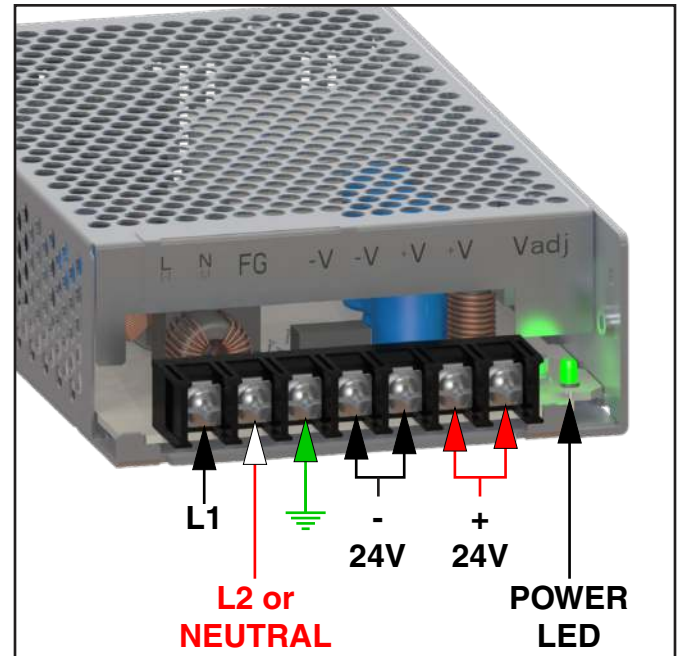
FIG. 23-2 SH POWER SUPPLY
