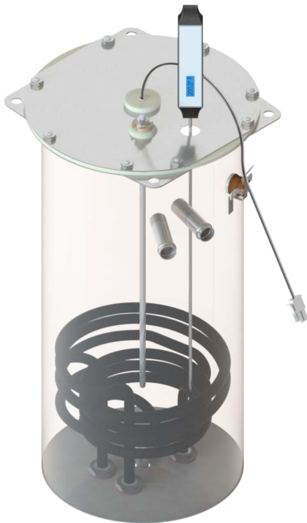
FIG. 20-1 CALIBRATE TEMP PROBE
