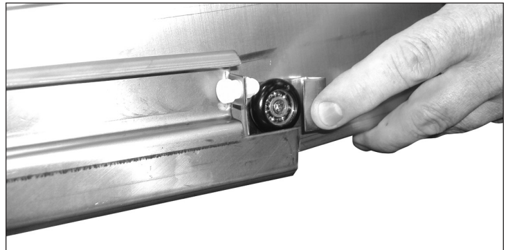
Fig. 4. Carefully lift the drawer from the channel slots.
