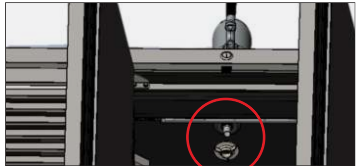
Fig. 1. Spill tray tube nut installation location.
