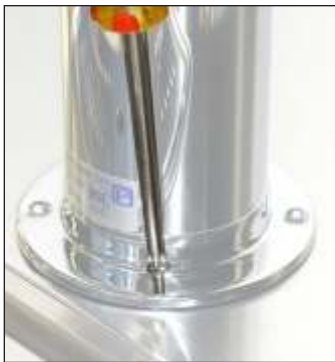
Fig. 5. Ensure the rubber gasket is between the countertop and draft arm.
