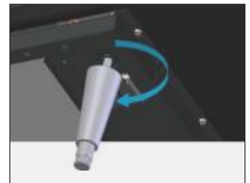
Fig. 4. Screw in the leveling legs.
