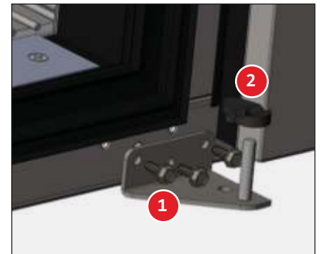
Fig. 9. Install the bottom hinge pin in its new location.
