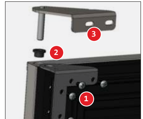
Fig. 7b. Top hinge component assembly.
