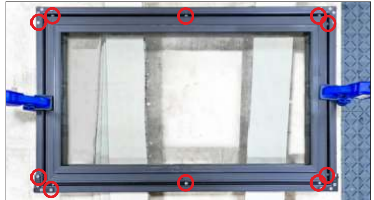
Fig. 7. Cabinet door predrilled hole locations.
