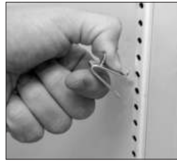
Fig. 1. Installing top tab of shelf clip.
