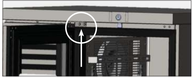
Fig. 1. Top hinge bolt locations.
