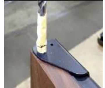
Fig. 9. Drill the 3/8" hole first. THEN drill the 17/64" hole.
