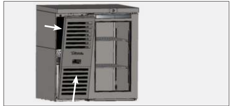
Fig. 2. Pull the grill forward before lifting up.
