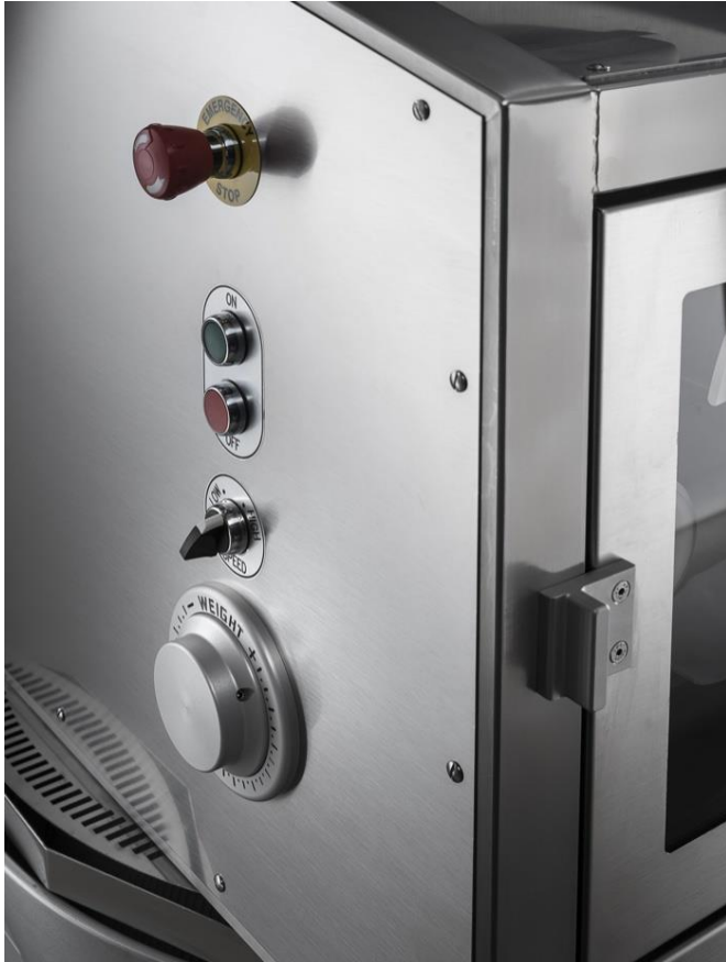
Emergency Stop, On / Off Buttons Speed Control and Weight Control
