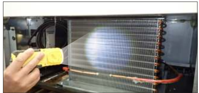
Fig. 3. Verify all blockages have been removed.
