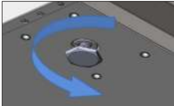
Fig. 2. Turn the leveling legs counterclockwise to raise the unit.
