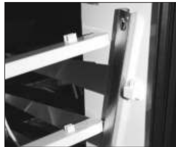
Fig. 8. Position the rear brackets over the rear notch.
