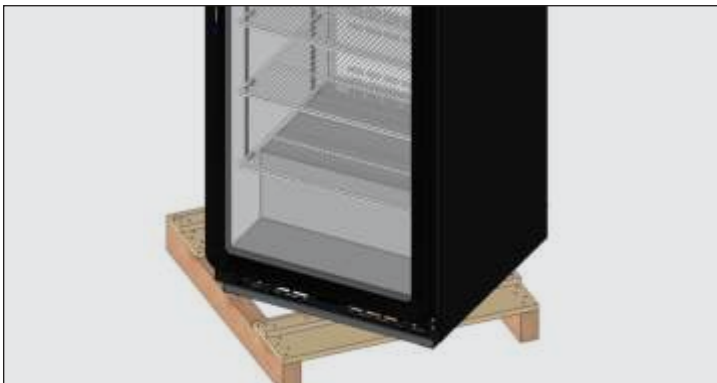
Fig. 4. Rotate the appliance on the skid. When lifting the appliance, do not use countertops, doors/drawers, or grills as lifting points.
