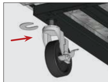
Fig. 9. Insert the castor shim(s). be sure to tighten the castor stem.
