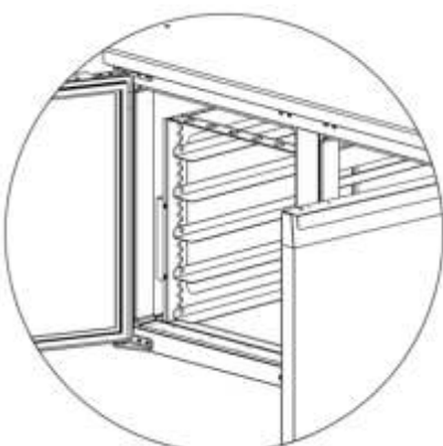
FIGURE 18C: Pan Slide Cage - Install Angle Slides
