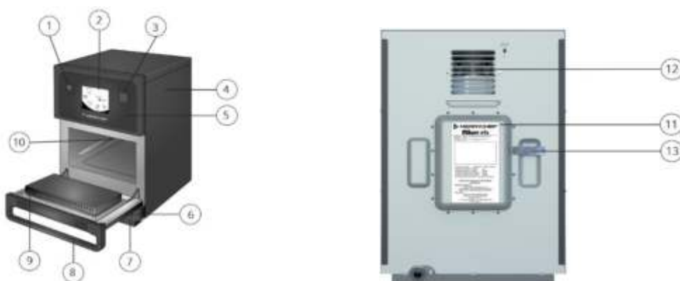
Figure 1.3: e1s front and rear views – parts and safety devices
