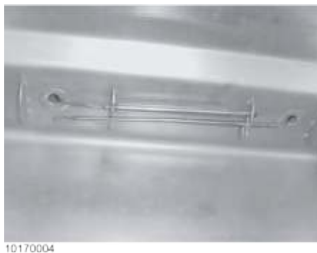
Figure 2-2 Thermostat Sensing Bulb - Gas
