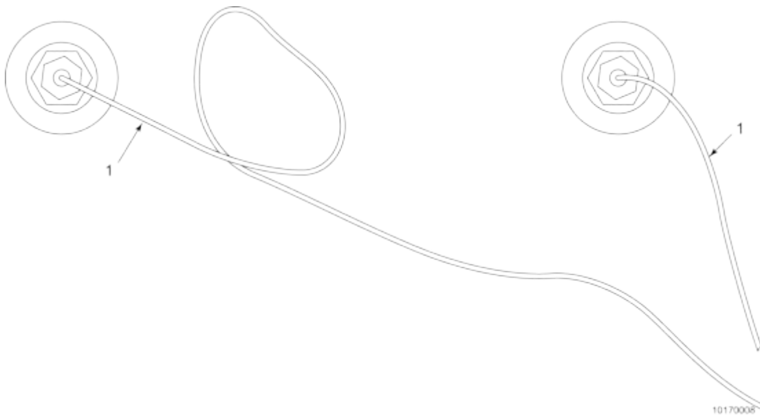
Figure 2-6 High Limit Capillary Tube - Gas
