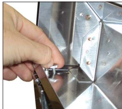
Fig. 2. Hold the rainshield open with the thumbscrews.
