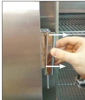
Fig. 3. Pull the hinge cover from the door hinge.
