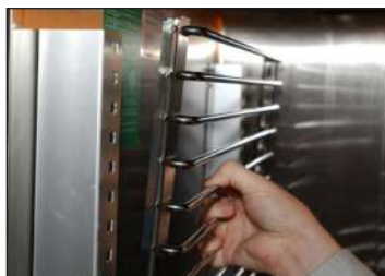
Fig. 7b. Installing kit #2 rod tray sides.
