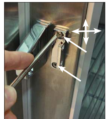
Fig. 6. Lock base screw locations. Move the base as needed.
