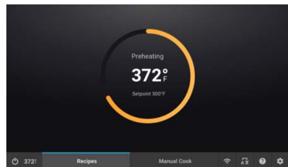
Figure 6: Oven Controls: OneTouch Preheat
