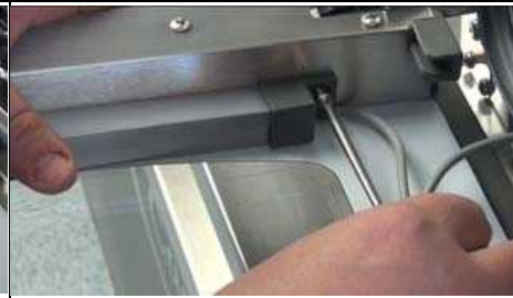
Fig. F 6) With Phillips head screwdriver, unscrew and remove both light cover brackets. Figs. E-F-G.
