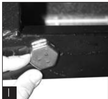
Back out leg levelers by hand, or with adjustable wrench.
