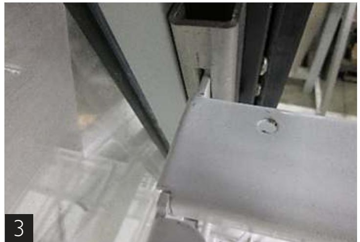
Light assembly installed on shelf support
